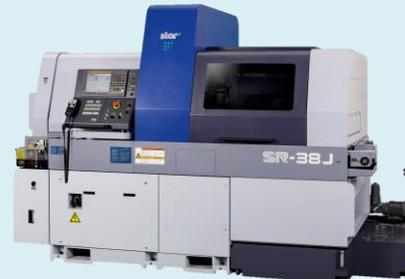
CNC Swiss Type Automatic Lathe
