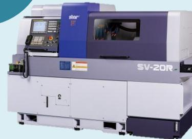
CNC Swiss Type Automatic Lathe
