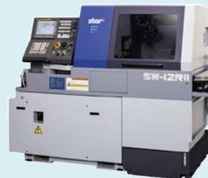
CNC Swiss Type Automatic Lathe
